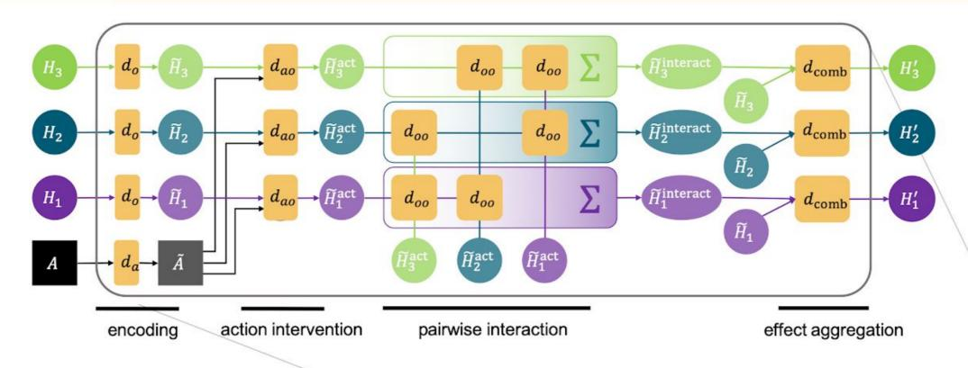
**Entity-Factorized Dynamics Model** The dynamics model independently evolves each entity state forward in time with the same functions by considering inertial and pairwise interactions between entities.
